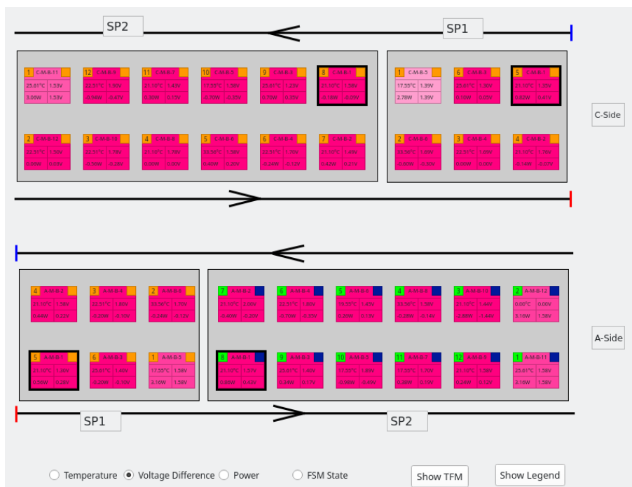
Figure 7.10: Quick test of the monitoring panel for a layer 3 longeron using the new module template, with the colour mapping toggle set to voltage differences.
