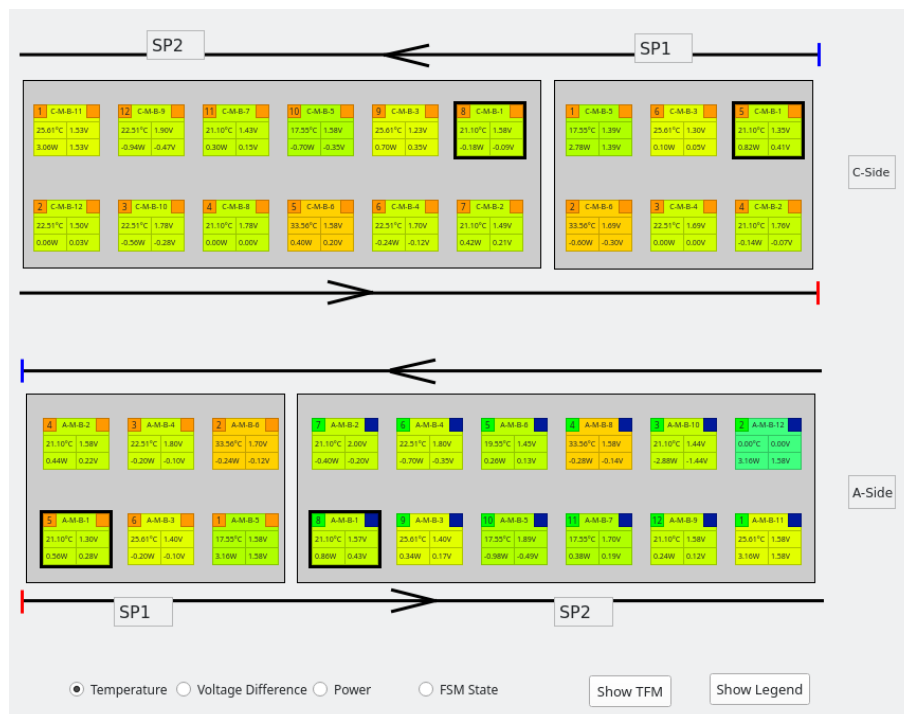
Figure 7.8: Quick test of the monitoring panel for a layer 3 longeron using the new module template, with the colour mapping toggle set to temperature.
