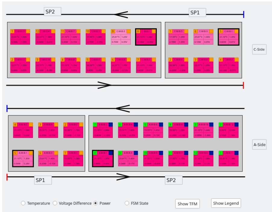
Figure 7.9: Quick test of the monitoring panel for a layer 3 longeron using the new module template, with the colour mapping toggle set to power.
